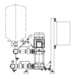
Inverter-controlled units with two vertical multistage pumps.
